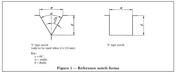
**4.6** The reference notch shall be formed by machining, spark erosion or other methods.
